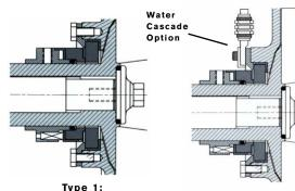
External Balanced Seal with Replaceable Mating Surface
