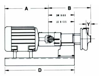
Note: Dimensions X, Y & B apply to pumps with clamp connection.
