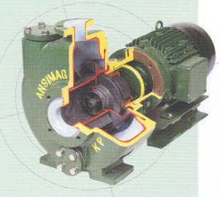
Developed to meet rising demand in the chemical handling industries for heavy-duty corrosive applications, the KP model is particularly effective in tank car/rail loading systems and waste chemical sumps. The internals are constructed of fluoropolymers and resist virtually every known chemical on the inside while rigid castings support heavy pipe loads on the outside.
