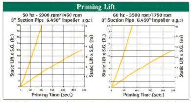
Priming Time will be reduced when smaller suction pipe is used. Priming Lift will be reduced as temperature of liquid increases.
