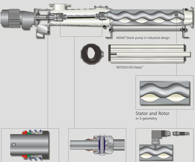
Shaft Seal Mechanical seal
