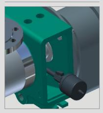
The Permanent Lubricator is used to support the sealing function of a shaft seal. This can be used for packed glands as well as mechanical seals fit with an additional quench ring. The lubricator provides a constant flow of grease into the quench ring, or lantern of the seal, against the pressure of a spring within the unit. If the pump is not run for any period of time the lubricator can be isolated with a valve. The unit is a robust metal construction and can be refilled.
