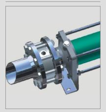
For the transportation of high viscosity media we recommend the installation of our ring dosing nozzle. The nozzle fits directly to the discharge connection of the pump and allows the injection of a boundary layer lubricant. Depending on the lubricant used the pressure loss in the discharge piping can be reduced by up to 70% in comparison to operating the system without any lubricant injection. By operating this system both the investment and operating costs are significantly reduced.
