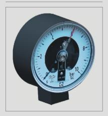
The pressure gauge displays the operating pressure. The gauge is isolated from the process fluid with a stainless steel diaphragm. With an adjustable pressure setting the pump will shut down when the maximum allowable pressure is exceeded. Suitable for low up to medium viscosities.
