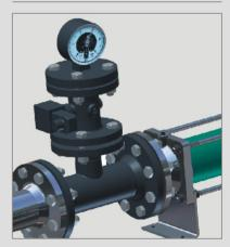
Display of operating pressure by a bourdon gauge. The gauge is isolated from the process fluid by an elastomer diaphragm. With an adjustable pressure setting the pump will shut down when the maximum allowable pressure is exceeded. Also available with a differential pressure on/off switch.
