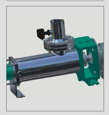
The flow sensing unit is used to protect a progressing cavity pump fitted with a stator against dry running. The unit senses the flow in the suction or discharge pipework. Should the flow drop below a predetermined level, indicating a dry running situation the unit will shut down the pump, thus preventing any damage.
