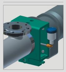
A quench pot is necessary when a shaft seal needs to be operated with a quench, but it is not required that the seal has a permanent flushing flow. So that dry running of the seal or crystallization of the pumped product can be prevented we recommend the installation of a quench pot.
