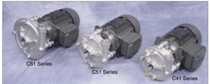
mal wear. These units also make use of our custom manufactured D3 dual face motors found on our T31, E41, and E51 turbine pumps, and feature a stainless steel shaft and a heavy duty front motor bearing. D3 Motors also feature UL and CE approvals. The C Series standard construction is investment cast 316 SS casings and impellers with Viton elastomers. Options - See below.
