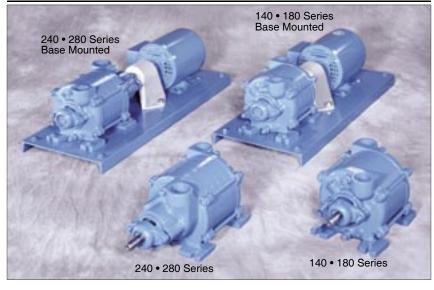
steel. Impeller is cast bronze, hydraulically balanced and self-adjusting for longer life. Sealed ball bearings are permanently lubricated for maintenance free operation. "O" ring gasketing is used to assure sealing and for ease of maintenance. Standard mechanical seals are rated for 230° F water operation. All units are flexible-coupled for easy service and motor flexibility. Pumps are 100% tested to guarantee performance prior to shipment.
