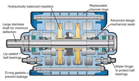
The 200 Series inducer style pumps are ideally suited to applications where available NPSH at the pump inlet is limited, such as boiler feed water deaerator service.
