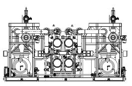
Self-priming, double entry, horizontal pump types
