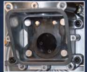
Four bolts release valve cover for service
